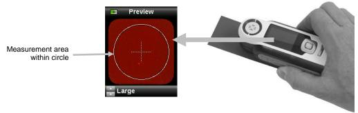
3. Hold the instrument steady and press the **Measure** button firmly and release. An audible "camera-click" sound indicates the start of the measurement. A progress bar appears at the bottom of the display to indicate the measurement status.
