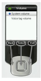
Screens that contain images of "arrows" indicate that the Up and Down sides of the Navigation control are used to adjust or page-through options, standards, etc.
