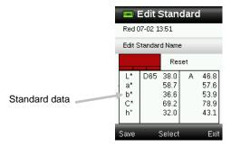
8. To enter a name for the standard, use the up or down sides of the **Navigation** control to select "Edit Standard Name" and then press the **Enter** (Select) button.
