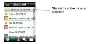
Press the up and down sides of the **Navigation** control to select the next available standard location.
