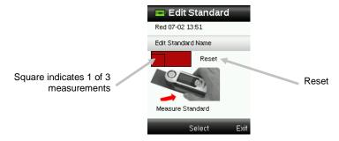
**Note:** If you do not want the current measurement to be used, use the **Navigation** control to select **Reset** and press the **Enter** (Select) button.
