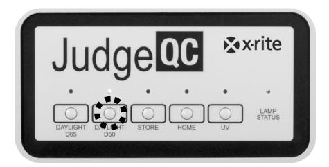
c) Switch off the main power behind the unit. The lamp status indicator is reset and will only resume counting from when the unit is next powered up.
