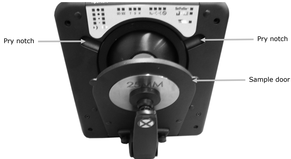
Figure 1. Opening the hinged sample door
