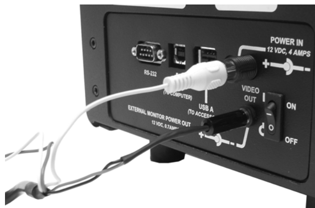
Figure 4. Monitor cable connections
