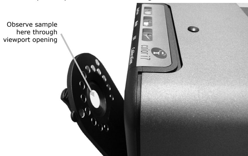
Figure 2. Observing the sample through the viewport opening
