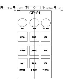
Step 6 - After 2nd pass complete, rotate strip and align it with the right guide so you can measure the Yellow field.
