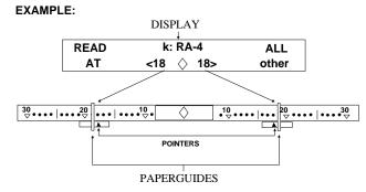
To move the paper guides to the desired location, lift-up on bottom slightly and slide left or right (see below).
