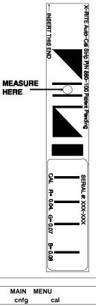
Step 3 - At Main Menu level, repeatedly press [p#] until "p3" is displayed. Press [cal] to activate calibration.
