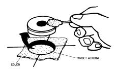
• NOTE: When cleaning the aperture always cover the target opening.
