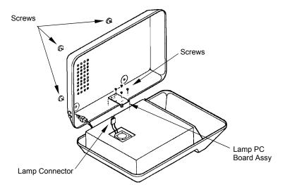
Figure 7. Lamp PC Board Access
