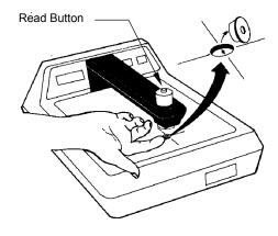
Figure 2. Aperture Removal
