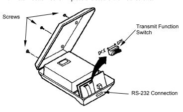
Figure 9. Transmit Function Switch Access
