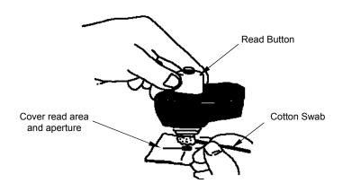
Figure 5. Cleaning Instrument Optics
