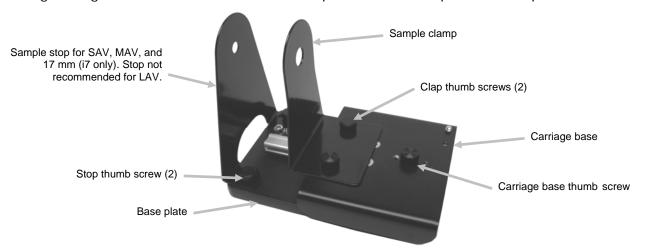
**Base Plate with Stop and Clamp Attached**
