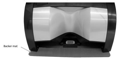
For best color measurement results, position the sample surface so that it is parallel (or flat) with respect to the instrument's four feet.
