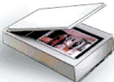
Creating a scanner profile requires scanning an IT8 target. You can scan the target using your scanner software and load the saved scan, or if you are using a Windows workstation with a compatible scanner, you can scan the target directly into MonacoEZcolor. The software will guide you through the process by prompting you to provide certain information and to perform tasks with your scanner.
