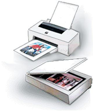
Profiling a printer requires using a reflective scanner as a measurement device. The procedure results in the creation of both an RGB scanner profile and a printer profile.
