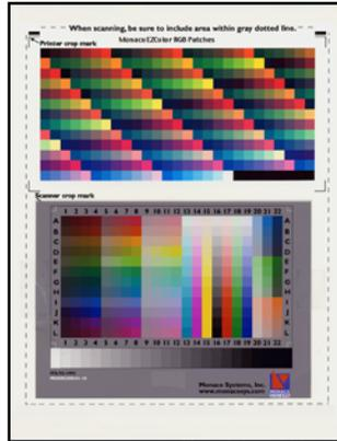
*IT8 target taped to Printer target before scanning*
