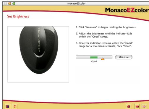
1. With the measurement device in position over its displayed outline, click **Measure**.
