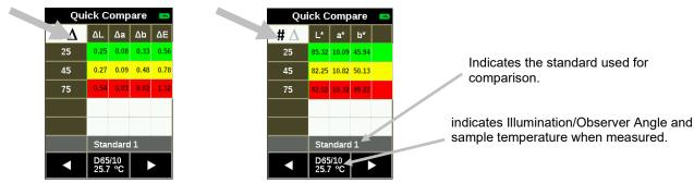
Data fields in tolerance appear green and red for out of tolerance. Data fields can also appear amber for a warning limit.
