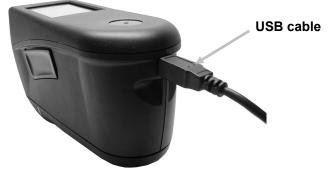
During charging, the instrument switches on and indicates charging with a "lightning bolt" in the battery icon. The instrument will not power off while plugged into the computer USB port, however, it will go into standby mode. This is indicated by a blue pulsing LED.
