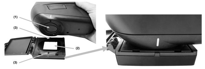
3. When ready, tap **Calibration** and then tap **Yes** to start calibration. Do not touch the instrument throughout the measurement sequence.
