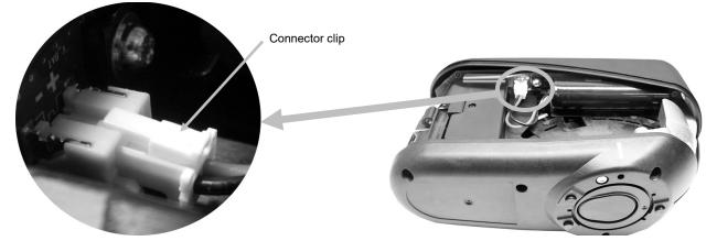
4. Insert the new battery pack into the clip and plug in the battery connector.
