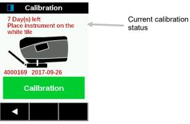
**NOTE:** If an error message appears after white calibration, try measuring the white tile again. If an error still occurs, clean the white calibration tile as explained in the Appendices. If the issue persists, perform Factory Reset in the Settings menu, turn the device off and on and repeat the calibration.
