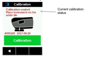
**NOTE:** If an error message appears after white calibration, try measuring the white tile again. If an error still occurs, clean the white calibration tile as explained in the Appendices. If the issue persists, perform Factory Reset in the Settings menu, turn the device off and on and repeat the calibration.
