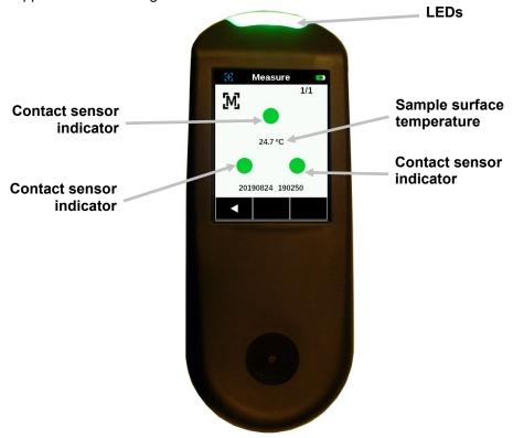
The multi-color LED located on the front of instrument provides visual feedback on the status of a measurement and contact sensor.
