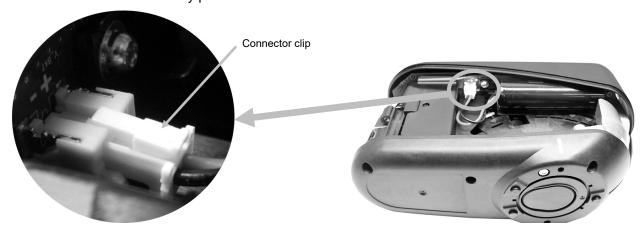
4. Insert the new battery pack into the clip and plug in the battery connector.
