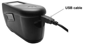
During charging, the instrument switches on and indicates charging with a "lightning bolt" in the battery icon. The instrument will not power off while plugged into the computer USB port, however, it will go into standby mode. This is indicated by a blue pulsing LED.
