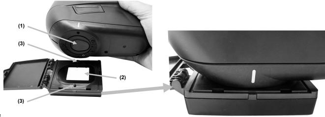
3. When ready, tap **Calibration** and then tap **Yes** to start calibration. Do not touch the instrument throughout the measurement sequence.
