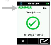
8. If the job was created on the instrument using the New Job feature, you can edit the name if desired. Tap on the Edit icon at the button of the screen and enter a job name using the virtual keyboard. Tap the Enter icon to save the job name.
