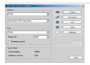
If you click on the **Maximum speed** check box, your spectrophotometer is set to a 57600 baud transfer rate. Do not select this option if your spectrophotometer is being used with a printer or other device having a lower transfer rate. Please refer to the operating instructions for the spectrophotometer.
