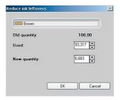
2. Click on the desired recipe and then on Select. The recipe will be converted into an ink leftover and added to the current assortment. In the Colorant selection window the original designation of the recipe will then be displayed in the Selected colorants field, marked with a \$ - sign.
