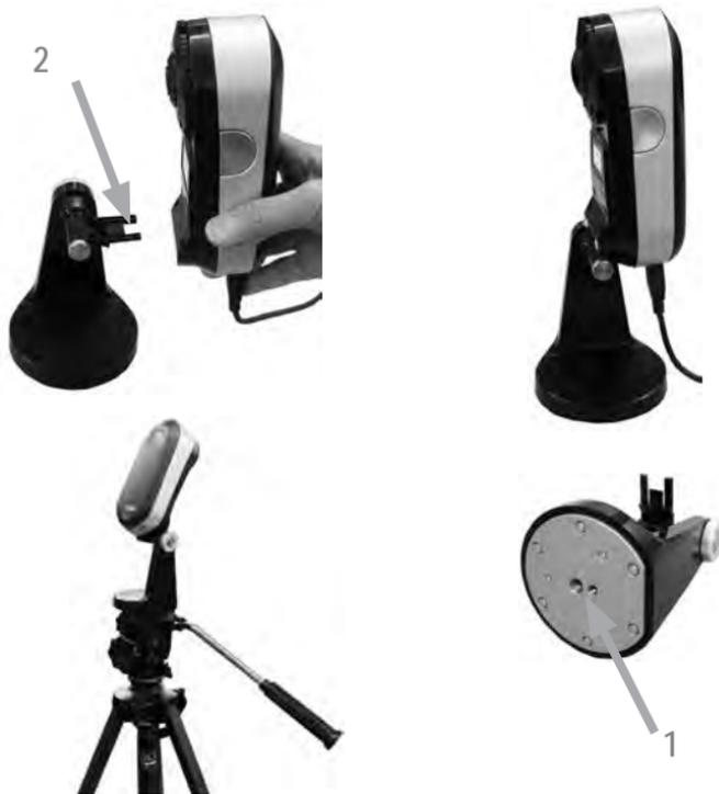
To prepare your i1Pro 3 device for projector measurements you can use the device on the tripod holder, or mount the tripod holder on a tripod with one of the two standard screws you supply (1). Next you need to mount the i1Pro 3 device on the tripod holder. Make sure that your device is calibrated and the status indicator is pulsating white before you mount the device.
