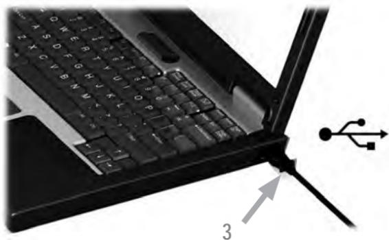
Before you can use your device or see its status, you need to install the software application on your computer. Please do not plug the device's USB cable into your computer until after you have installed the software application.
