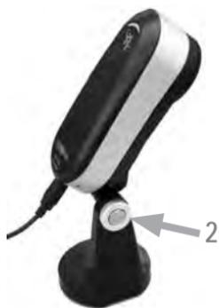
Setup the i1Pro 3 device for projector measurements.
