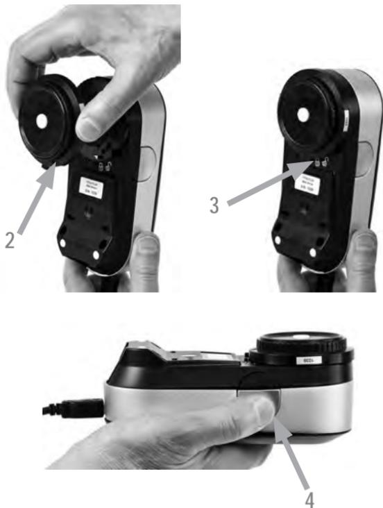
Before you start measuring, please attach the ambient light measuring head on the limiting aperture of the i1Pro 3 device. If you own multiple devices make sure that the serial number on the ambient light measuring head matches the serial number of your i1Pro 3 device. The ambient light measuring head can also be used in conjunction with the tripod holder.
