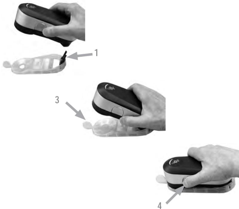
To prepare your i1Pro 3 device for spot measurement you need to mount the i1Pro 3 device on the positioning target. Make sure your device is calibrated and the status indicator is pulsating white before you mount the device. Refer to the user guide of your measurement software for further details on the spot measurement process.
