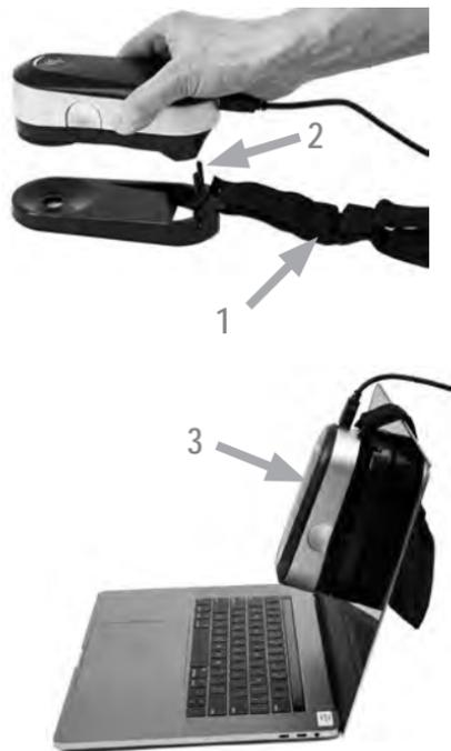
To prepare your i1Pro 3 device for a display measurement you need to mount the i1Pro 3 device on the display holder. Make sure your device is calibrated and the status indicator is pulsating white before you mount the device.
