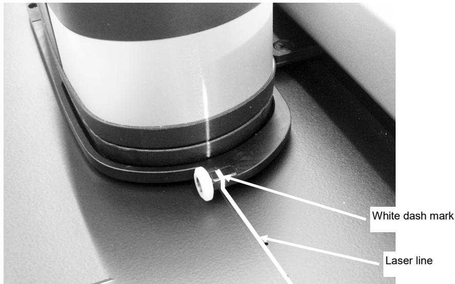
2. Place the edge of the press sheet at the white line (1) in front of the scanning trolley.
