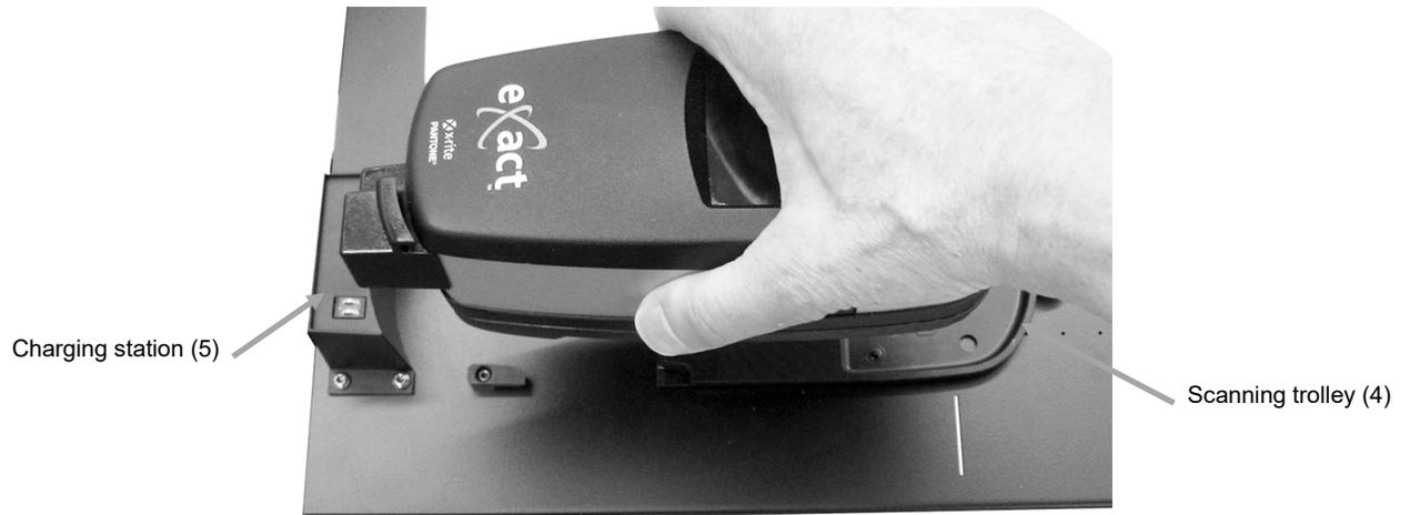
7. Secure the eXact to the scanning trolley by rotating the locking arm (6) counterclockwise until it stops. This holds the instrument in place during scanning.
