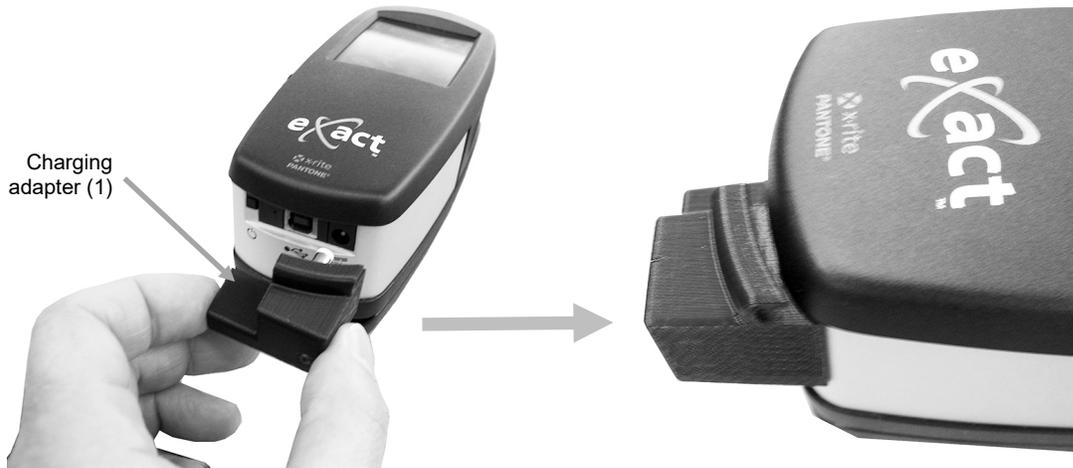
**NOTE:** If the Bluetooth function is not used, route the USB for the eXact instrument in the channel at the top of charging adapter. This will help prevent the cable from interfering with the charging station and track during operation. This USB cable is separate from the eXact Auto-Scan system USB cable that was previously installed. Plug the square end of the USB cable into the back of the instrument. Plug the USB cable into an available port on your computer.
