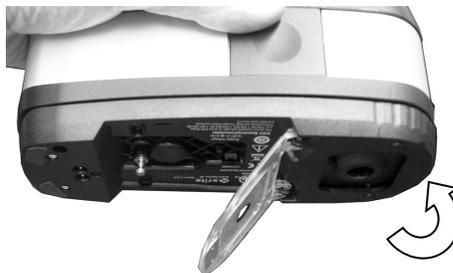
3. Position the target window over the sample to measure. The opening should be completely filled with the sample color.
