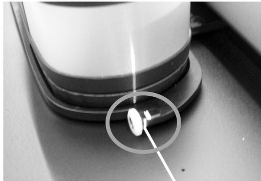
3. If the laser line is to the back of the white dash mark, rotate the alignment wheel adjustment upward to center the laser line on the white dash mark.
