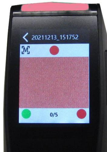
Example 2: Two pressure sensors are not contacting, and the measurement cannot be triggered
