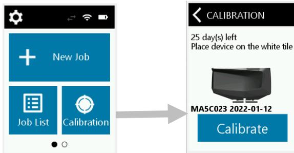
2. Separate the calibration reference and position the device measurement port over the white tile as shown in the image below. Make sure that the two alignment pins insert into the openings in the white tile reference. **Note:** The pins will only insert in one direction. Make sure you have the device aligned correctly. Disconnect the device from the USB cable while calibrating the device
