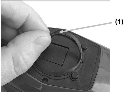
2. Orientate the new light seal over the recessed area around the measurement port.
