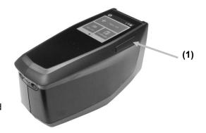
When powered-up, the device goes through a diagnostics test. The status LED and screen illuminate white, followed by a splash screen before the main screen. This startup sequence will take a few seconds to complete.
