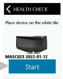
4. After the white tile calibration is completed, place the device on the camera test target as explained in the Calibration Mode section and tap the **Start** button.
