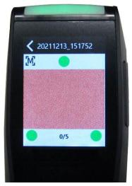
Example 1: All pressure sensors are contacting correctly, and a measurement can be triggered
