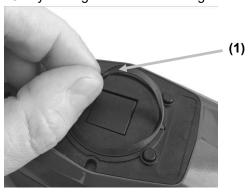
2. Orientate the new light seal over the recessed area around the measurement port.
