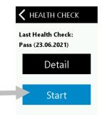
3. Place the device on the white tile as explained in the Calibration Mode section and tap the Start button.
