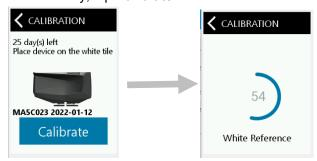
4. After white tile calibration, remove the device from the white tile and position the device measurement port over the camera test target as shown in the image below. Make sure that the two alignment pins insert into the openings in the camera test target. **Note:** The pins will only insert in one direction. Make sure you have the device orientated correctly.
