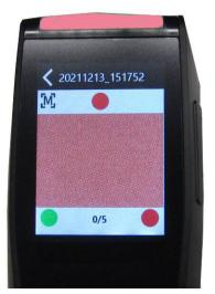
Example 2: Two pressure sensors are not contacting, and the measurement cannot be triggered
