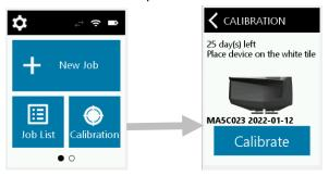
2. Separate the calibration reference and position the device measurement port over the white tile as shown in the image below. Make sure that the two alignment pins insert into the openings in the white tile reference. Note: The pins will only insert in one direction. Make sure you have the device aligned correctly. Disconnect the device from the USB cable while calibrating the device
