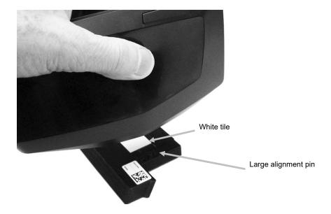
3. When ready, tap Calibrate. Do not touch the device throughout the measurement sequence.
