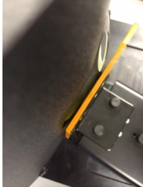
**Transmission holder with sample at the sphere (total measurement) for 25 mm, 17 mm, 10 mm, and 6 mm, measurements**
