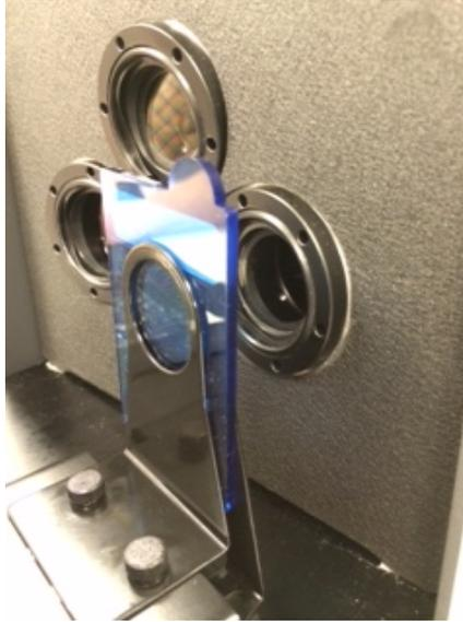
7. Once properly position, tighten the thumb screws and close the transmission cover.
