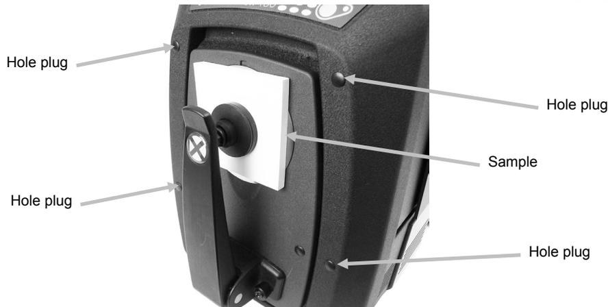
6. Use the computer screen or the drop down door to view the sample and adjust the sample measurement targeting area.
