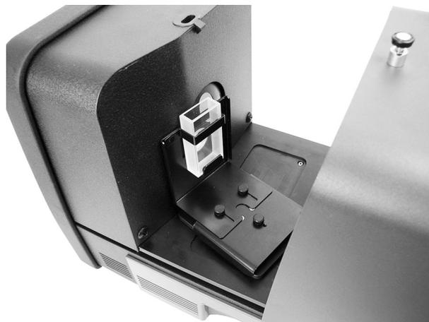
5. Initiate the measurement by selecting "Measure Standard" or "Measure Trial" from your software application, or press the Standard or Trial button on the front panel.
