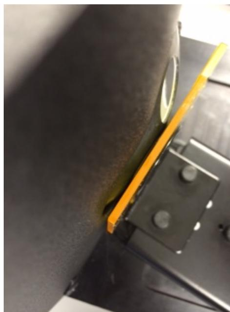
9. Once properly position, tighten the thumb screws and close the transmission cover.
