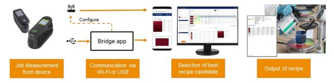
The Auto SC web app supports job measurements sent via Wi-Fi from the MA-3, MA-5 and MA-T5 devices. Jobs can also be sent through USB connection to a PC using the Bridge app for the same devices and the MA91.
