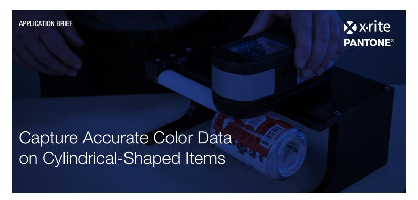
X-Rite's Cup and Cylinder Solution combines the eXact or Ci6x handheld spectrophotometer with a sample-positioning arm to hold a cylindrical-shaped sample at the correct height and angle for color measurement.
