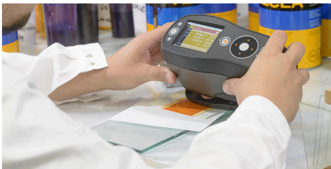
X-Rite Ci61: Measurement of a wide range of sample types for fast, accurate paint matching
