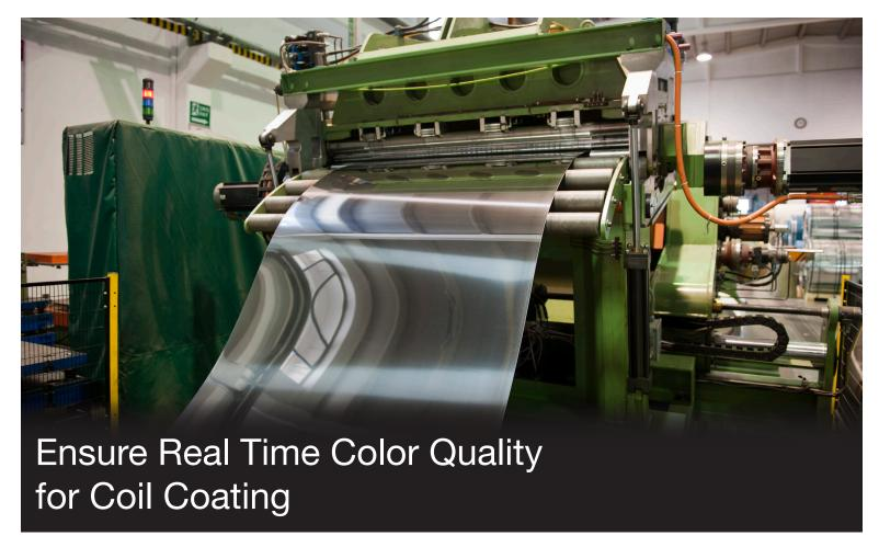
Coil coating paints metal in sheet form for superior, durable results in much less time. However, any shift in color or gloss on a fast-moving production line can quickly create a lot of waste. An inline color control solution can monitor color quality and ensure consistency in real time to avoid costly rework.
