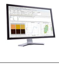
**Color iMatch Professional:** Ideal for anyone formulating color for plastics applications, this premium configuration includes the full gamut of features: quick, accurate color analysis, the ability to optimize every formula for cost and color accuracy, an integrated quality control module, and the ability to build or edit colorant databases.
