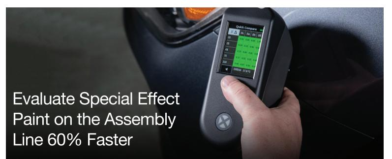
The MA-5 QC multi-angle spectrophotometer, along with EFX QC software, improves color evaluation accuracy as well as tracks data for process improvement on assembled automotive parts.
