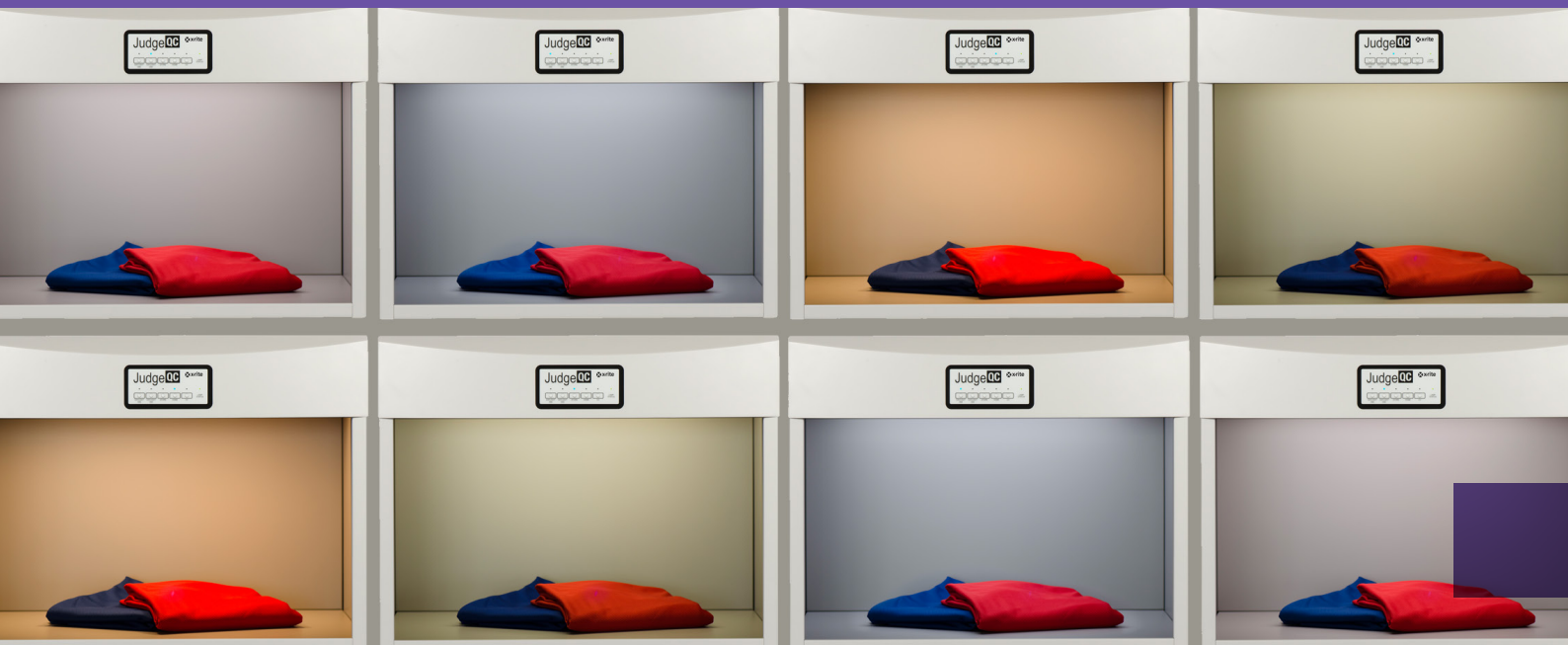
▲ PICTURED: With 5 light sources the Judge QC will help you evaluate standard to samples and batch-to-batch color variation.
