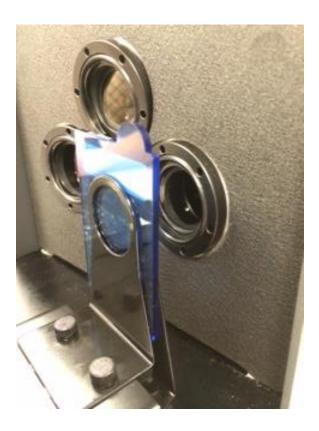
The sample is held in position using a fixture with a stop plate on the lens side of the sample, and a spring loaded clamping plate on the side of the sample away from the lens.
