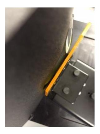
Care should be taken to properly align this fixture so that the stop plate is positioned flush and tight against the opening in the sphere. When setting up for measurements, do not tighten the thumb screws in the fixture until the stop plate has been positioned tight against this opening.
