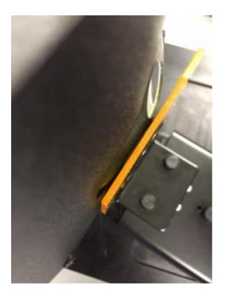
When doing the total transmission measurement the sample is held in position using a fixture with a stop plate on the sphere side of the sample, and a spring loaded clamping plate on the side of the sample away from the sphere.
