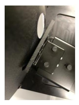
**NEVER** use the black trap for black calibration when performing total transmission calibration.
