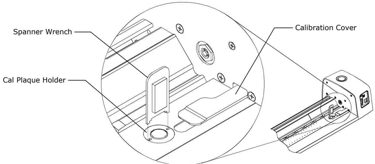
15. Remove the old cal plaque holder by turning the wrench counter-clockwise.
