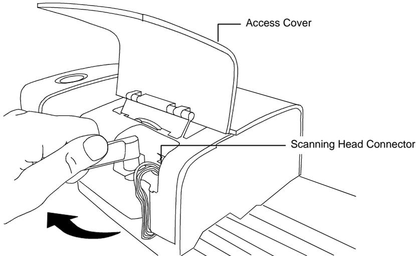
6. Lift up under the front edge of the scanning head and tilt it back to expose the bottom.
