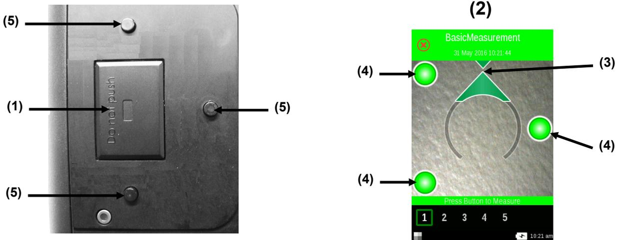
3. Gently rock instrument until all three positioning indicators (4) in the display screen turn green. This indicates that all three pressure sensors (5) are activated and a measurement can be taken.
