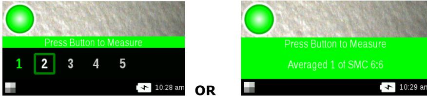
5. Position the instrument on the second sample area as explained in Instrument Positioning. Hold the instrument steady and press a **Measure** button or tap the screen.
