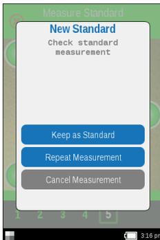
11. After **Keep as Standard** is tapped, the instrument goes into targeting mode. Position the instrument on the sample area to measure as explained in Instrument Positioning.
