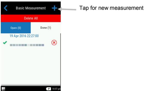
3. The instrument goes into targeting mode. Position the instrument on the first sample area to measure as explained in Instrument Positioning.
