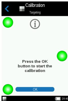
**NOTE:** If an error message appears after white calibration, try measuring the white tile again. If an error still occurs, clean the white calibration tile as explained in the Appendices.
