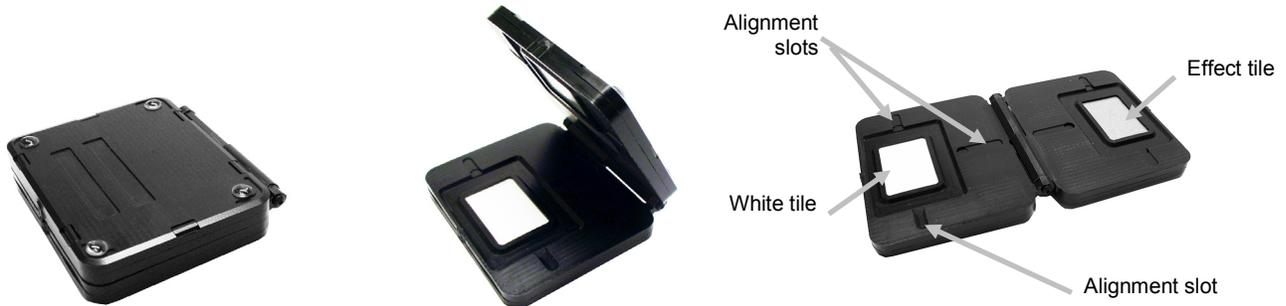
Lay the calibration reference flat. Position the instrument on the calibration reference over the tile so that the three pressure sensors around the measurement port align with the slots in the calibration reference, and the white lines align. This ensures the instrument is properly positioned over the white tile or effects tile.
