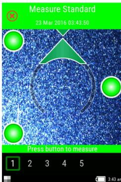
6. Hold the instrument steady and press a **Measure** button or tap the screen to initiate a measurement.
