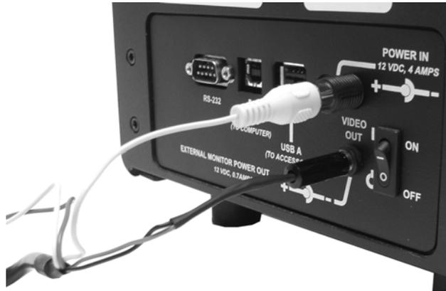
**Figure 4. Monitor cable connections**
