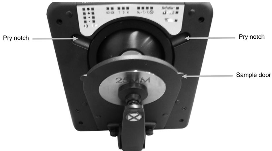
**Figure 1. Opening the hinged sample door**
