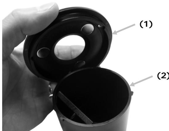
2. Look inside of the black trap to reference how the trap glass is positioned. This is important to remember when it comes time to reinstall it after cleaning.
