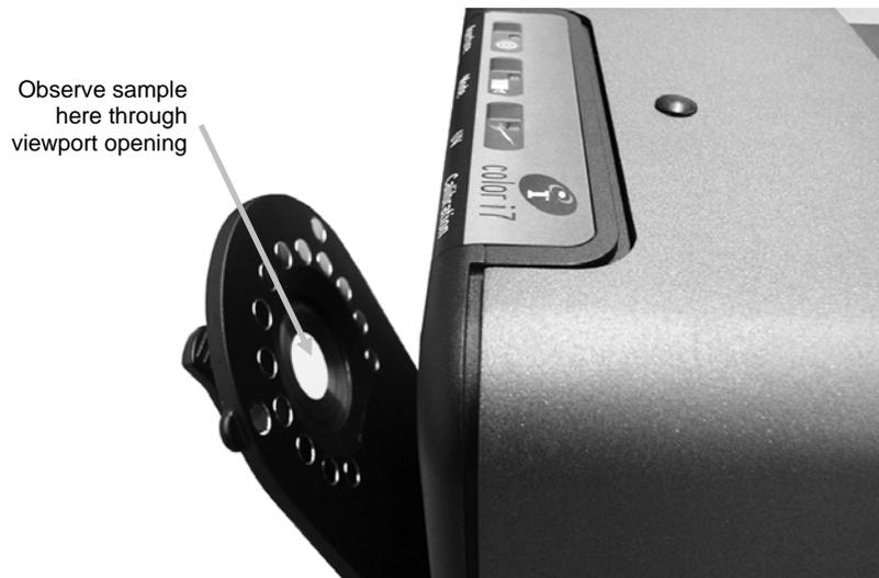
**Figure 2. Observing the sample through the viewport opening**
