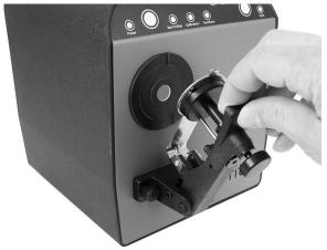
3. Pull the knob back and insert the color sample between clamp and retainer. Make sure the sample side you wish to measure is facing the sample port.
