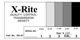
5. Recalibrate the densitometer following the Den calibration procedure, but replace the "hi entered" calibration value with the new "Dot cal" number generated in step 3.
