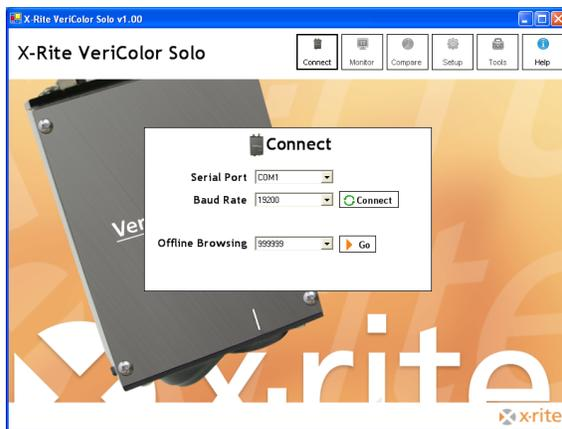
Communication is established by selecting the known COM port using the **Serial Port** control and baud rate using the **Baud Rate** control. After selecting **OK**, the Monitor screen opens.
