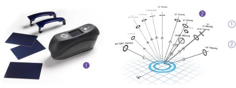
Capture spectral measurements of special-effect paints or coatings.
